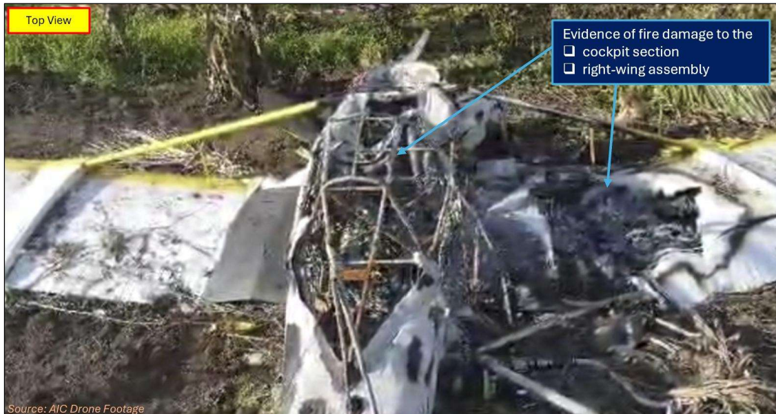
Figure 4. Evidence of post-impact fire at the accident site.
