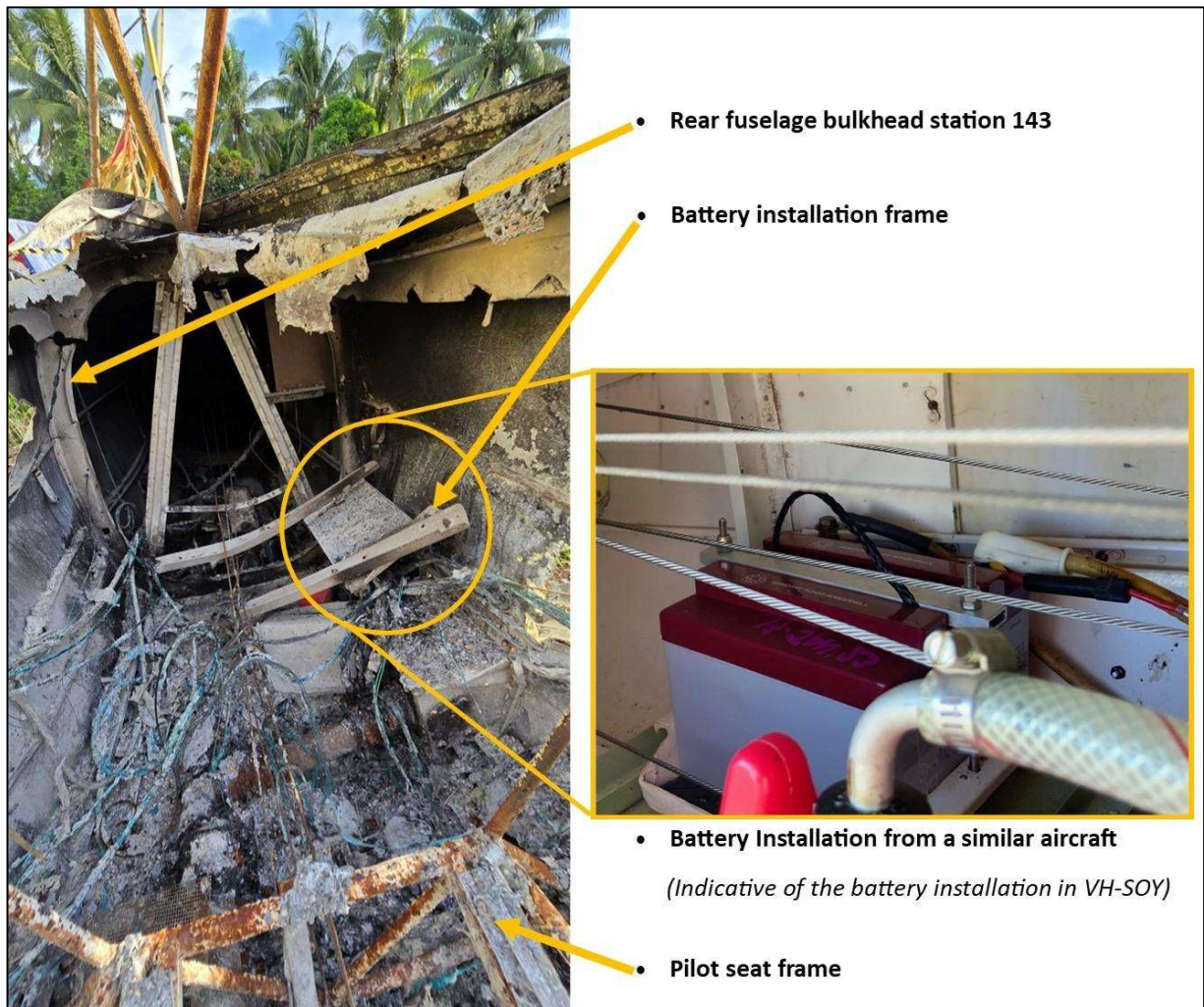
Figure 8. Rear fuselage showing battery installation area.
