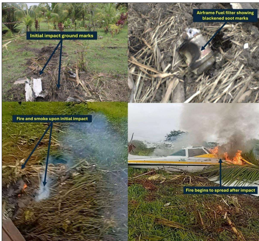
Figure 7. Initial ground marks and fuel filter showing blackened soot marks.
