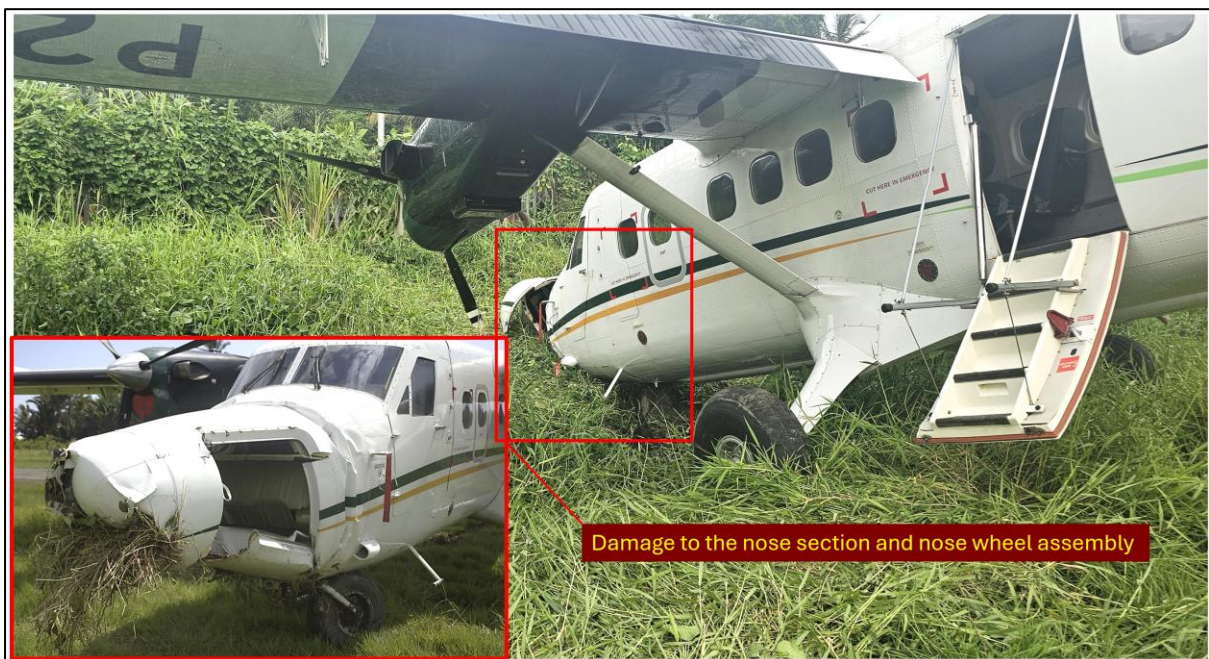
Figure 4: Overview of damage sustained by the aircraft
