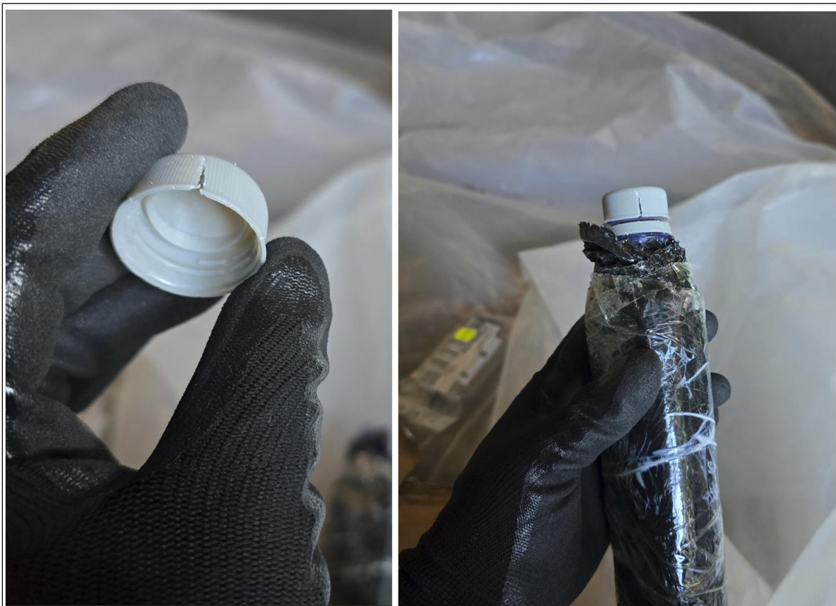
Figure 9: Empty bottles with broken lid from which the Spill occurred
