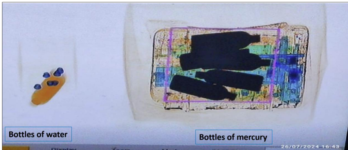
Figure 6: Images of re-scanned shipment in comparison to scanned bottles of water (Source: Air Niugini Ltd)
