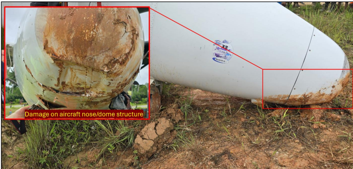
Figure 13. Damage to the nose cone/dome structure.
