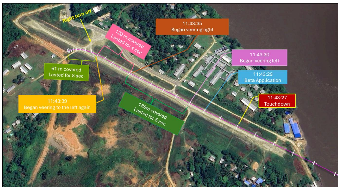
Figure 4. Aerial view of the airstrip and P2-BBM track from touchdown to final resting position.
