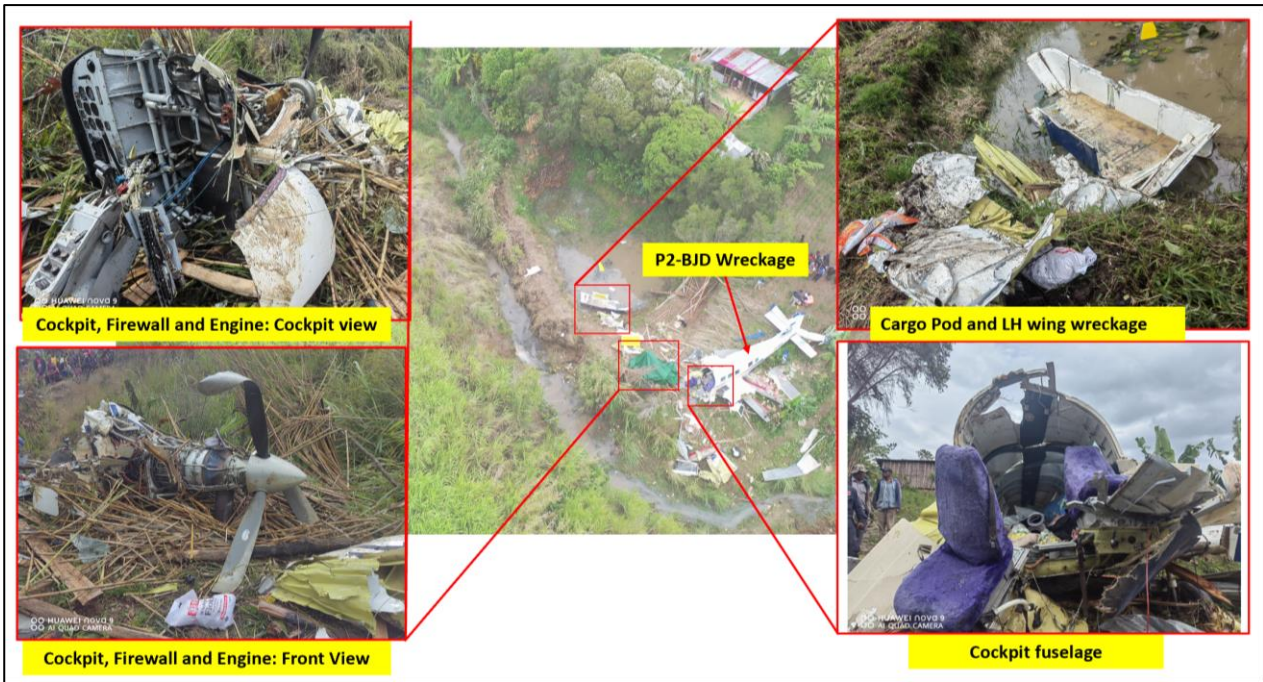
Figure 14: Wreckage distribution after second impact
