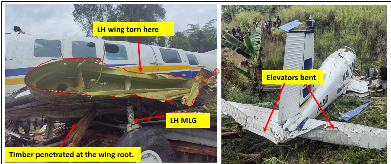
Figure 16: Damaged LH Wing and Elevator
