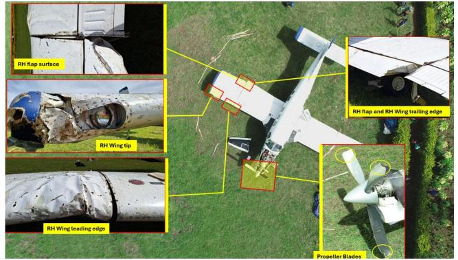
Figure 5: Overview of the damage sustained on the aircraft
