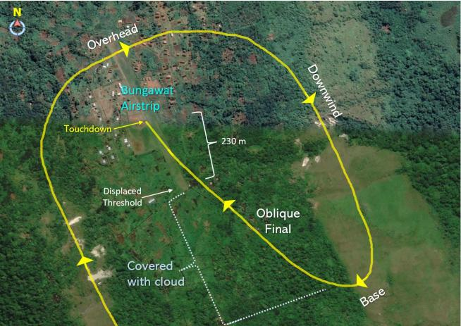
Figure 3: P2-NCA estimated overview of the circuit (Source: V2 Track recorded data and pilot interview)
