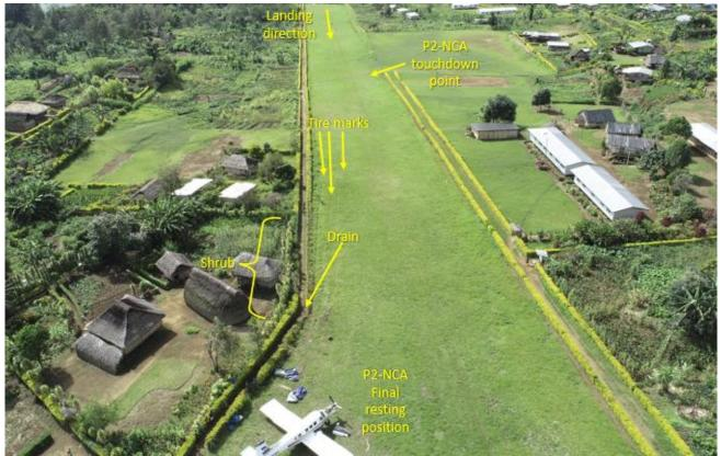
Figure 4: Overview of P2-NCA from touchdown to the final resting position
