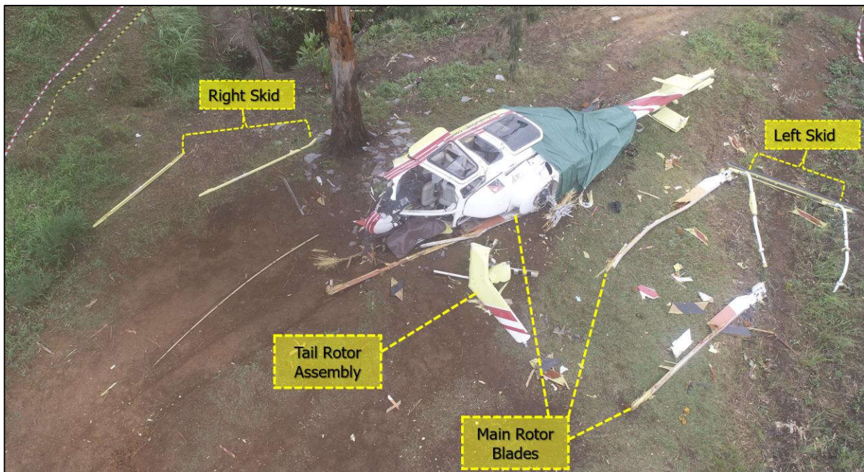
Figure 7: Overview of the damages sustained by P2-HSN
