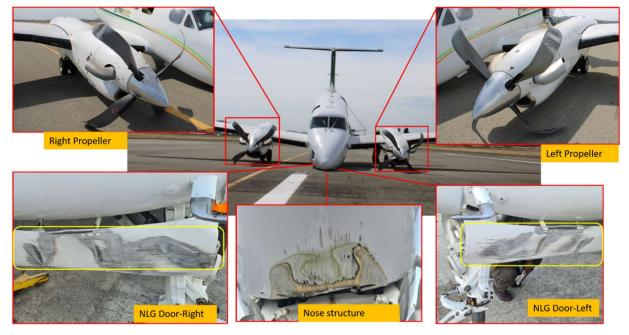
Figure 3: P2-JAU observed damage at occurrence site
