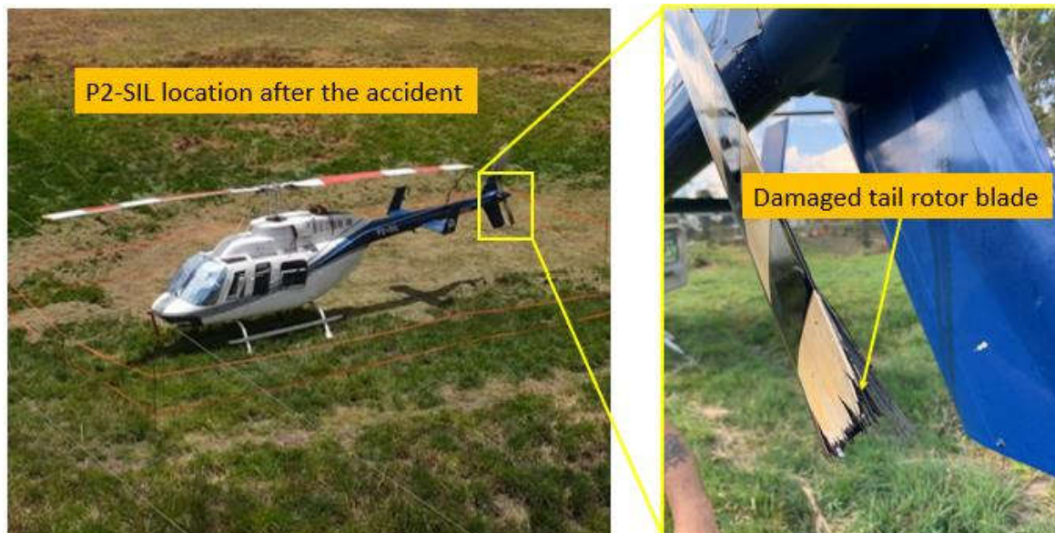
Figure 3. Damage sustained to the tail rotor blade.
