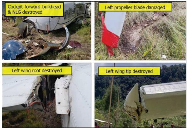
Figure 4 Damage sustained by P2-ASM
