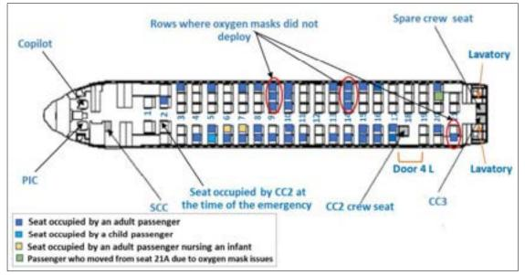
Figure 8: Cabin layout including crew and passenger seating arrangement.
