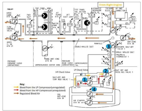
Figure 3: Bleed air schematics for No. 1 engine.
