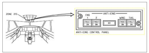
Figure 4: Anti - icing panel
