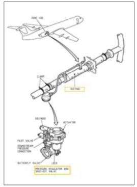
Figure 5: Engine anti-icing components
