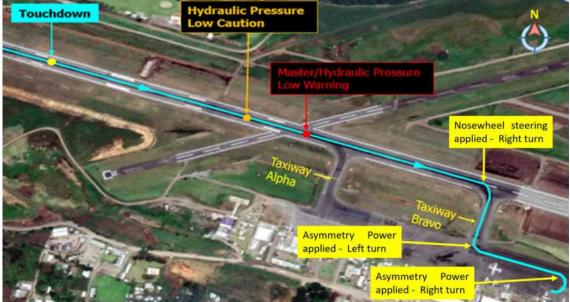
Figure 3: Alerts activated during landing roll.
