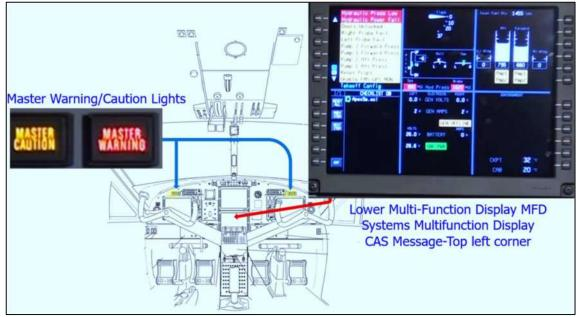
Figure 5: Crew alerting system display.
