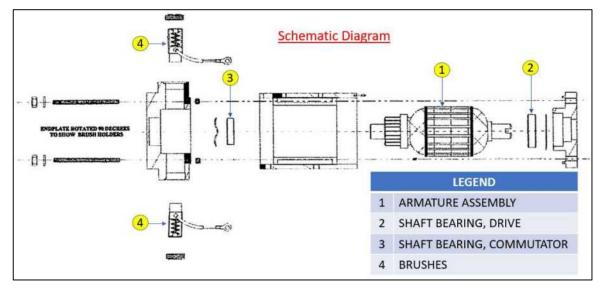
Figure 7: Electric motor schematic diagram.
