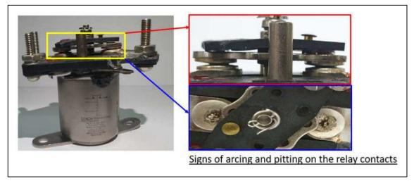
Figure 6: Relay removed from aircraft during post-occurrence maintenance.
