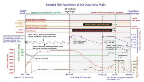
Figure 8: FDR Recorded parameters of the occurrence flight from take-off to touchdown.
