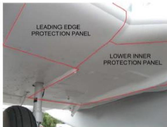
FIGURE 4 LOWER WING SURFACE (SHORT RANGE WING)
