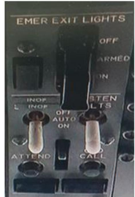
Figure 2: P2-PXE Cockpit Overhead Panel Emergency Light switch during the approach<sup>3</sup>
