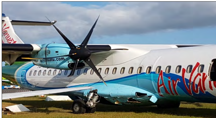
Figure 3: AV71 Right-side fuselage post impact damage
