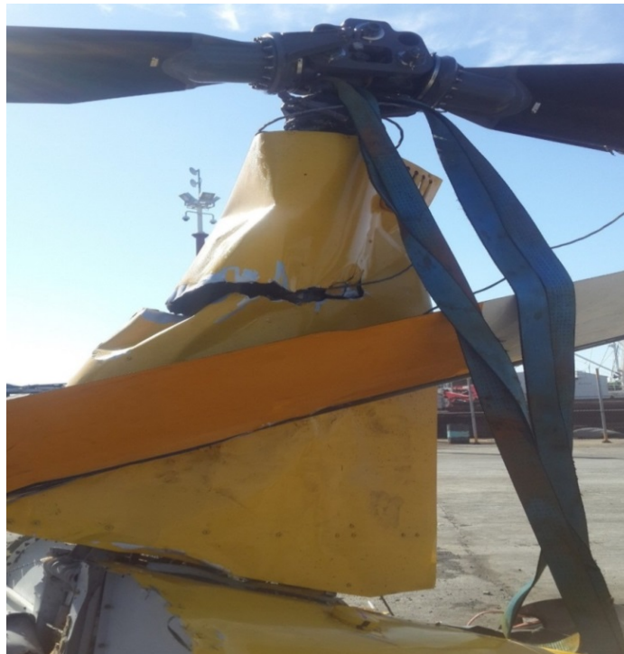
Figure 2: Wire Strike on the main rotor mast
