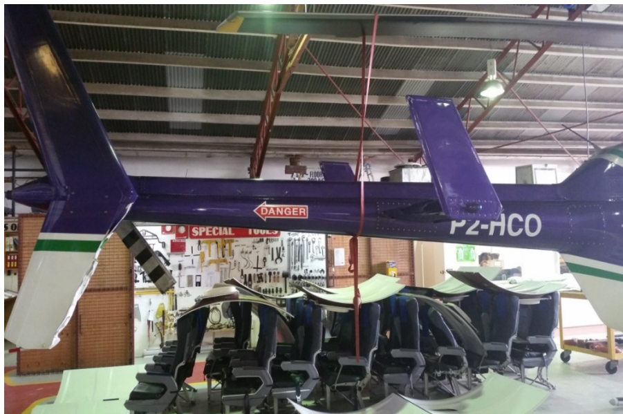
Figure 2: Damaged lower section of the vertical stabilizer
