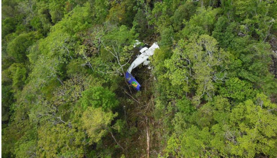
**Figure 6: Wreckage of KSF and impact trail**
