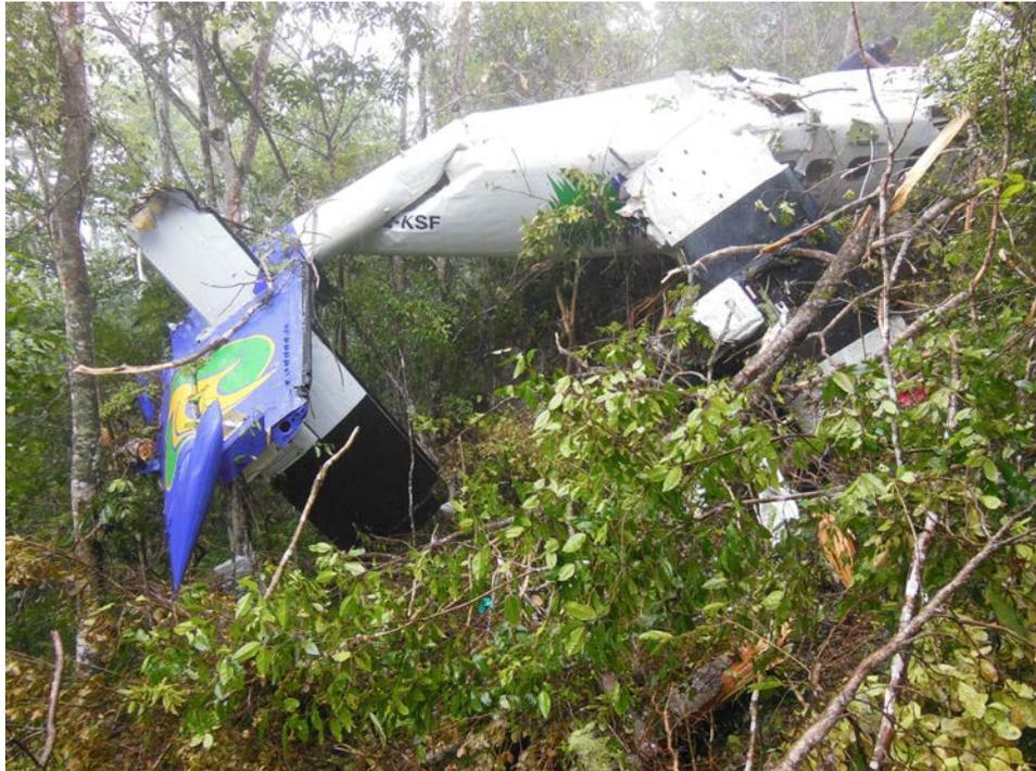
**Figure 8: Wreckage of KSF showing empennage hanging**
