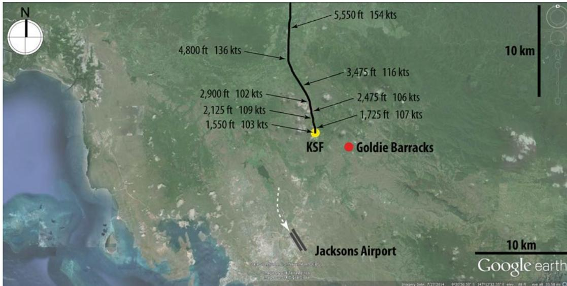
**Figure 2: Final part of the track taken by KSF; the dotted white arrow shows the approximate path to be flown from a left base position onto runway 14 right**
